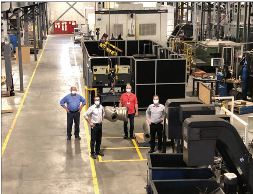
A segment of Velan's new cell layout to assemble large valves in Granby, Canada. Velan installed 25 manufacturing cells in Montreal, Granby, and India as part of the V20 transformation process.
