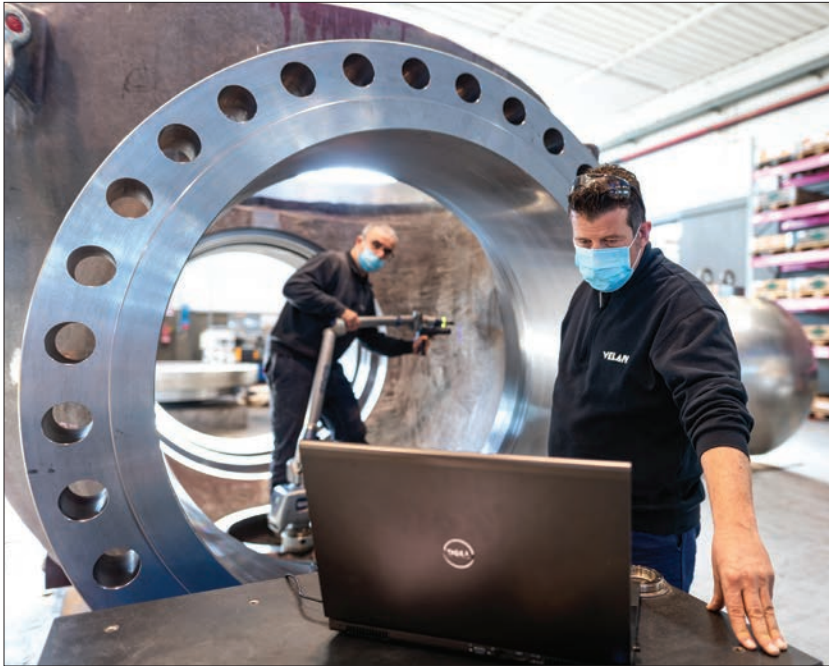
Velan ABV employees perform NDT and dimensional tests on a 52" ball valve using a ScanArm and 3D digitalization software to maximize the efficiency of the process.
