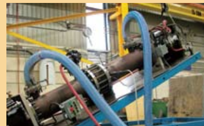
During testing, wafer check valves were cycled both vertically and, as seen here, horizontally.
