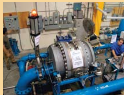
Qualification testing of a 34" titanium triple-offset butterfly valve in Velan's R&D lab. The valve had no leakage over the 10,000 cycle test.
