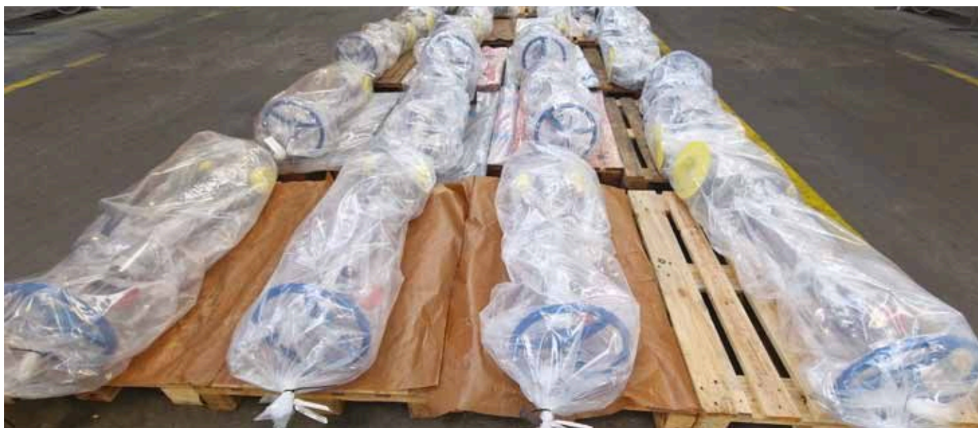
Oxygen cleaned valves ready to be shipped. Photo credit: Velan
