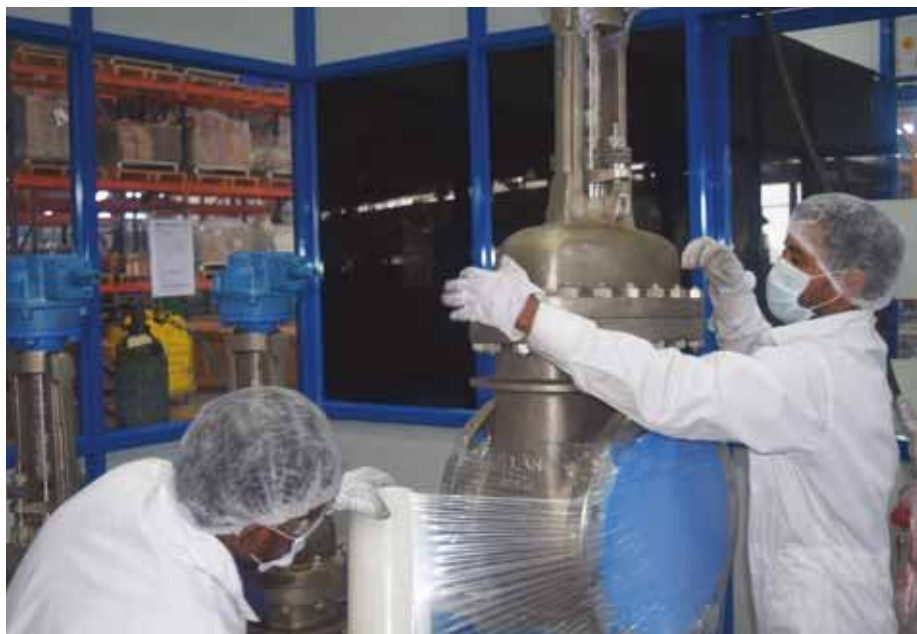
Oxygen cleaned gate valve. Photo credit: Velan
